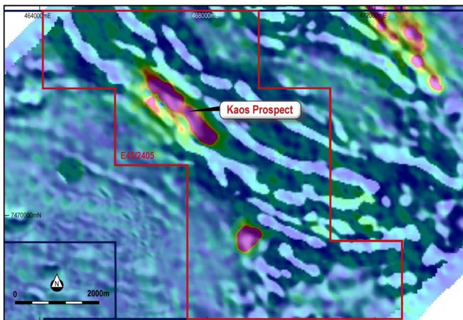
Figure 1: The Kaos Prospect is a 2.2km long by up to 250m wide Airborne EM conductor.
